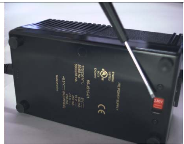
Figure 3.4-2: Bottom view of power supply showing voltage selection switch (220V)
