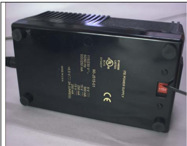
Figure 3.4-1: Bottom view of power supply showing voltage selection switch (115V)
