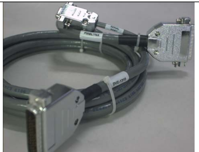
Figure 2.2-6: 10ft. interface cable, with 18" RS232 pigtail
