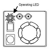
Switch the camera on by pressing the POWER button on the rear panel of the device. Observe the operation display (LED). If the camera is properly attached, the LED will flash **red-green** for approx. 3 minutes. During this time, the system is cooled down to a temperature of between -11 and -15 degrees Centigrade (5 degrees Fahrenheit).
