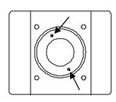
It may be necessary to adjust the back focal length. If the camera cannot be focused to infinity.
