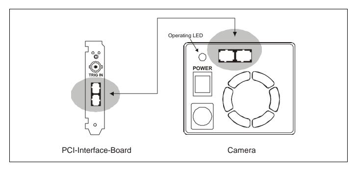
**Caution!** Avoid kinking or bending the cable over a sharp edge. This will break the core and destroy the cable.
