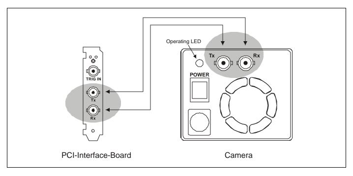
If other than delivered cables are to be used, make sure they have an impedance of 500. The maximum cable length for proper operation is 10m.
