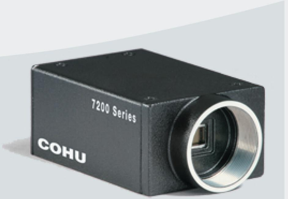
The Cohu 7200 Series is a small CMOS monochrome camera with FireWire interface with the size, features, and specifications that give it maximum productivity and economy. It operates in a non-interlaced (progressive scan) VGA format with full frame readout at up to 50 frames/second at 8-bits per pixel. It is IIDC 1.30 (DCAM-II) compliant and compatible with a Cohu graphical user interface (GUI) and SDK, as well as third-party software packages.
