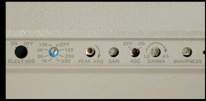
An easily removable trim plate allows access to the following sidepanel controls: Electronic Iris ON/OFF, Eight-Step Shutter Timing, ACG Peak/Average, Gain, AGC ON/OFF, Gamma, Black Level.
