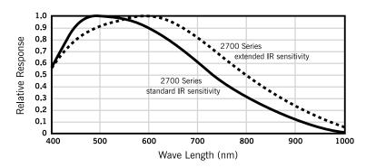
The extended IR sensor option of the 2700 Series provides increased low light sensitivity.
