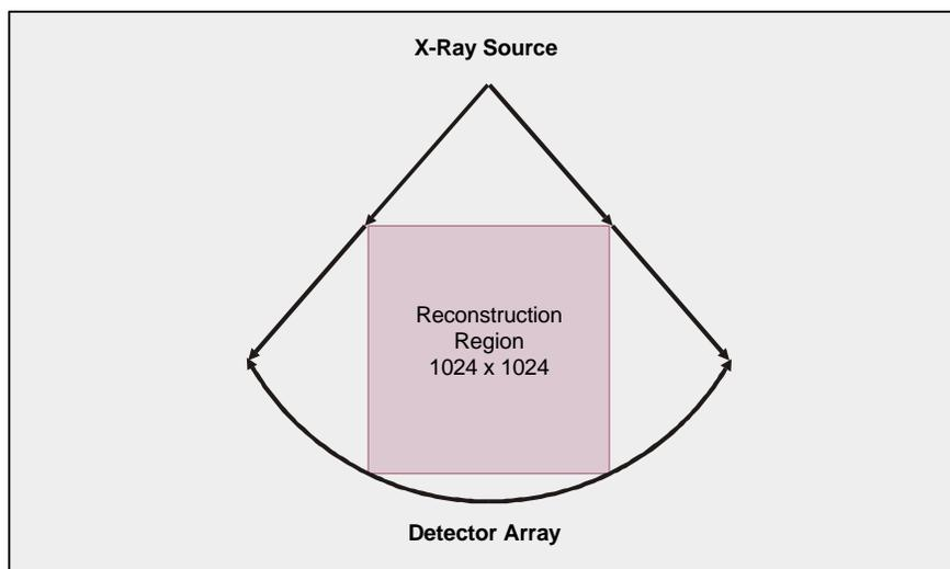
Figure 1: Relation of the region of reconstruction to the x-ray source and detector array.
