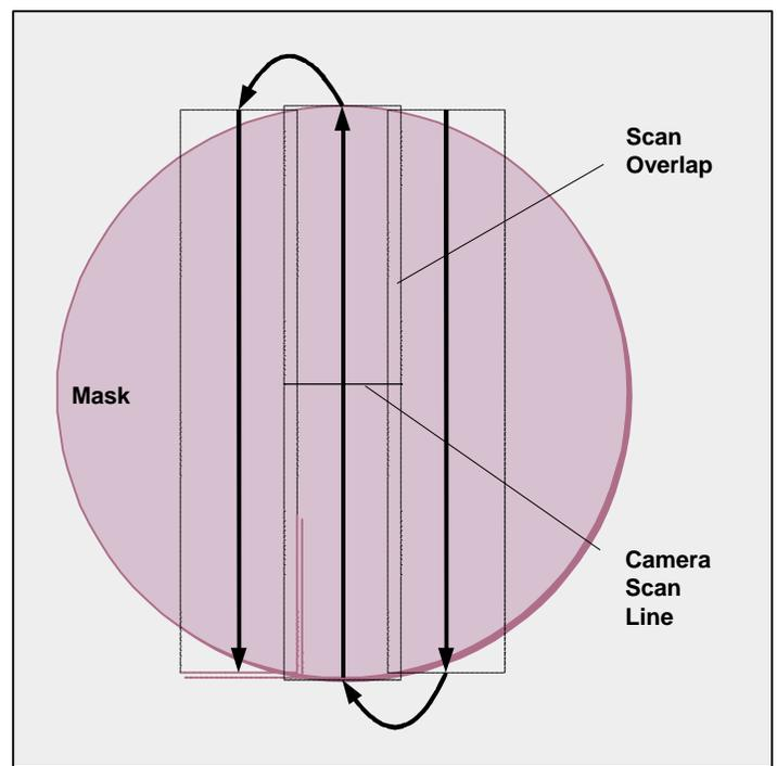
Figure 2: Diagram of imaging path.
