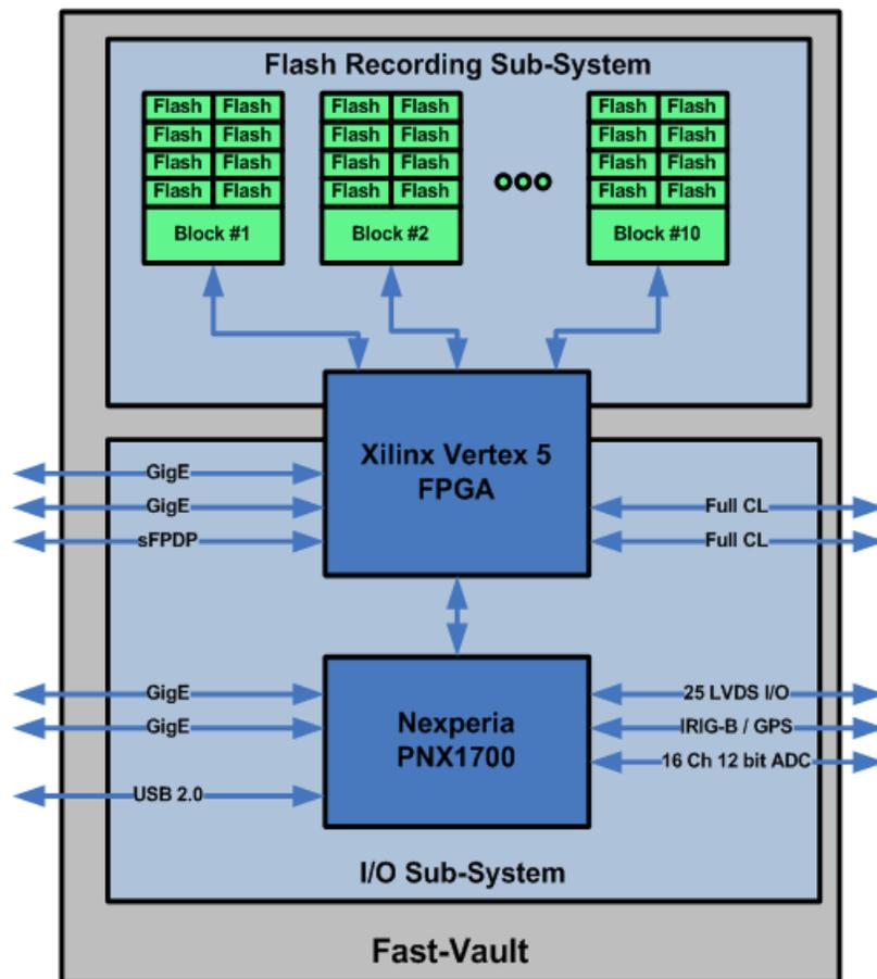
**BLOCK DIAGRAM OF THE FAST-VAULT**
