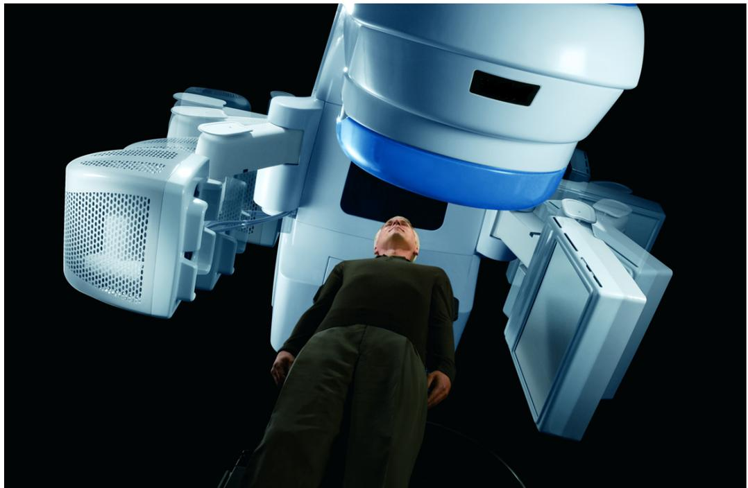
**PRECISION TECHNOLOGY:** This radiation oncology machine translates digitized data into extremely accurate, identifiable images; locates the tumor; then precisely aims radiation beams to kill it with minimum tissue damage.
